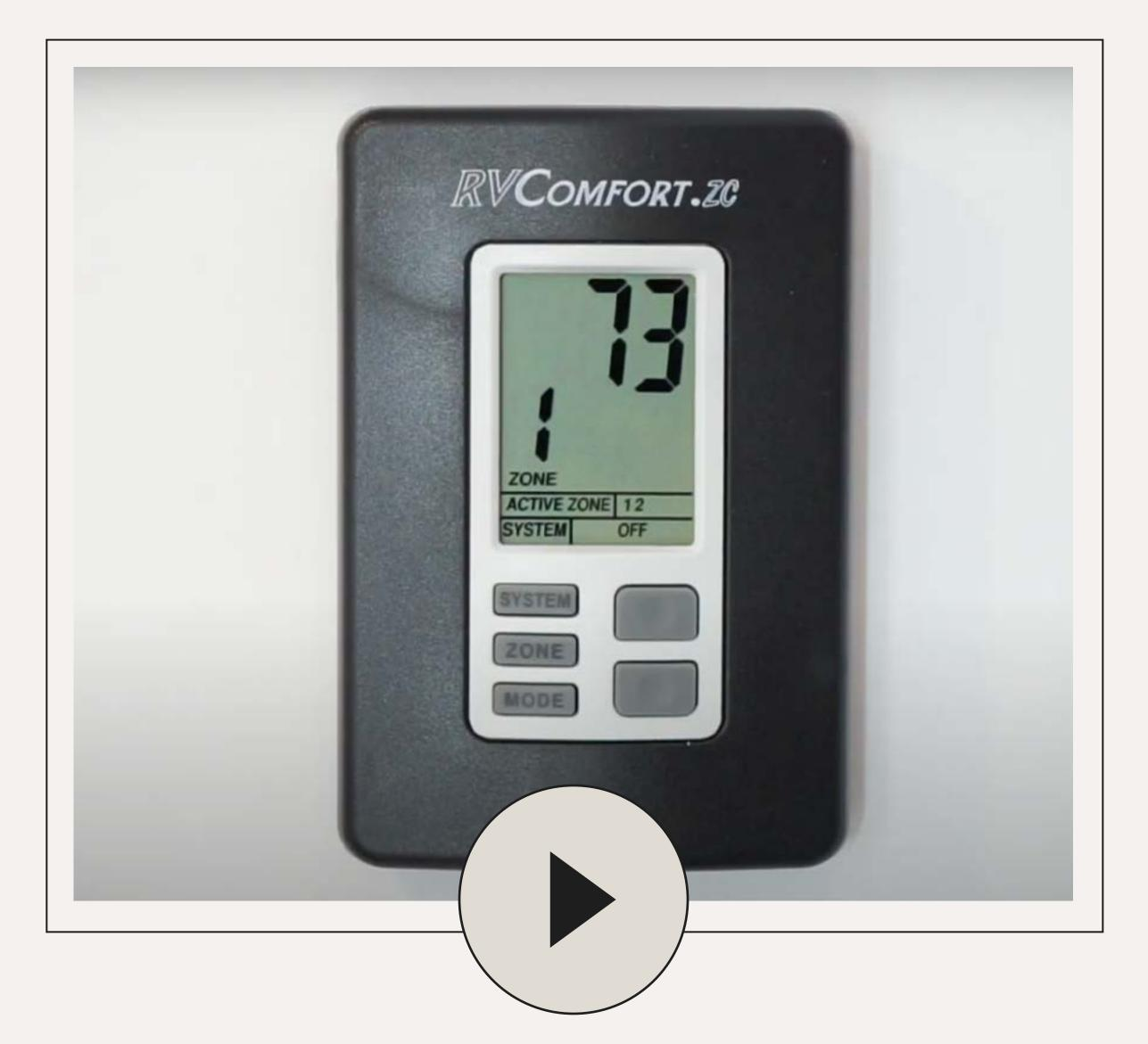
If you do not have wall heaters, your thermostat is located by the kitchen sink. **For heating,** press the system button until it says heat, then press the mode button until it says heat and gas, then adjust the temperature to your desired level. Please do not set temperature above 73 on heat / gas. **For air conditioning,** press the system button until it says cool. Then press the mode button until you see the snowflake symbol. Adjust the temperature to your desired level. No lower than 68
